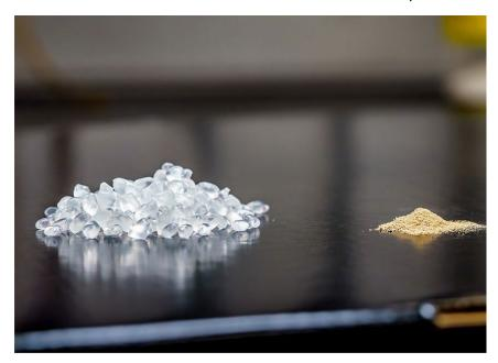
The biodegradable "living plastic" is made by combining thermoplastic polyurethane (TPU) pellets (left) and Bacillus subtilis spores (right) that have been engineered to survive the high temperatures used to produce the plastic.
