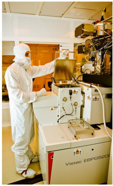
Ryan Anderson, a process engineer for the Nano3 facility in the Qualcomm Institute, prepares to remove a sample from the Vistec EBPG5200 electron beam writer.
