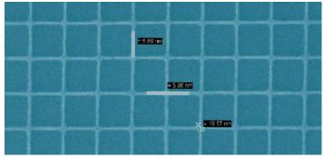
Colorized micrograph of an electron beam-written grid pattern demonstrating < 8 nm resolution capabilities of the EBPG5200.
