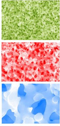
Nanofoams made from porous silica, with an average pore size of a few microns, seen at the 50-micron, 20-micron and 5-micron scale. Engineers are developing nanofaoms that disperse the force of an impact over a wider area than conventional foams.
